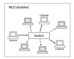
Figure 7-1. Without MLD, multicast traffic is flooded to all ports.
